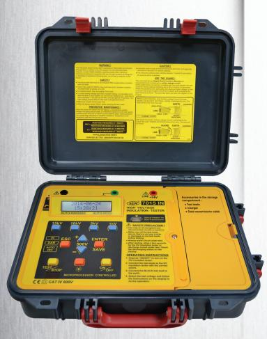
Insulation test voltage up to 15kV.
